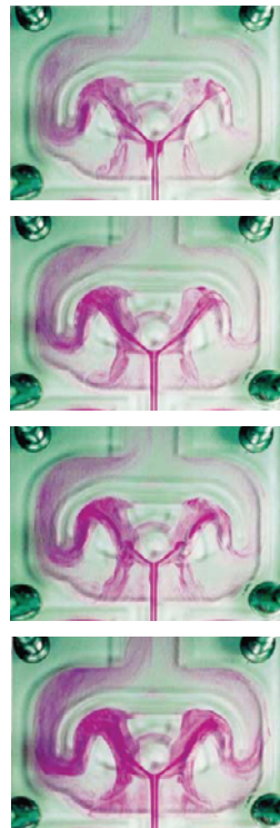
Fig. 11. Steady symmetrical flow of target oscillator with round target (Type D) in pulsating flow.
